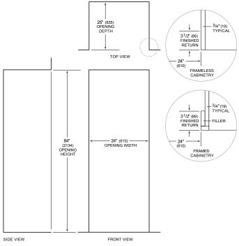
NOTE: 31/2" (89) finished returns will be visible and should be finished to match cabinetry
