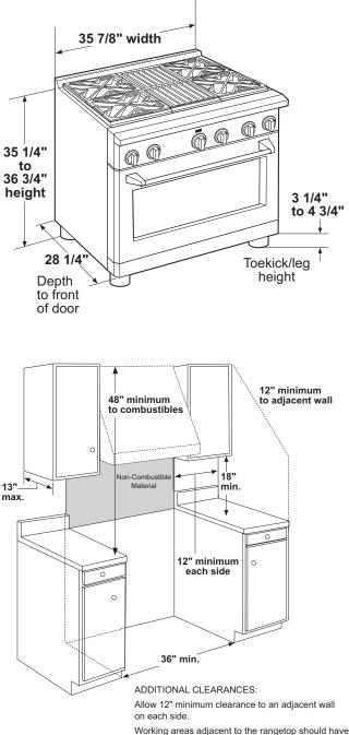
Working areas adjacent to the rangetop should have 18" minimum clearance between countertop and the bottom of the wall cabinet.
