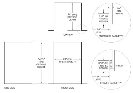
NOTE:  $3^{1/2"}$  (89) finished returns will be visible and should be finished to match cabinetry.
